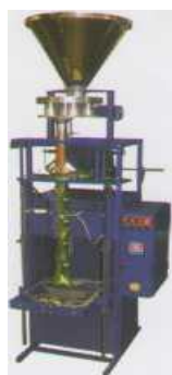
AF-35-OB automatic weighing-and-packing machine with a volumetric dosing unit
