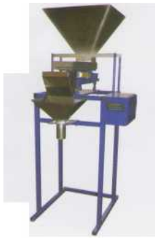
VD-1 weighing dosing unit
