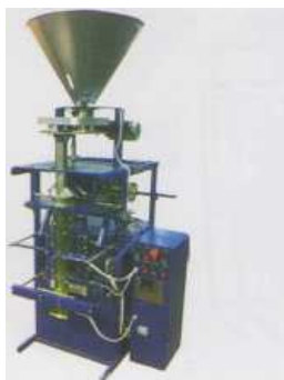
AF-45-OB automatic weighing-and-packing machine with a volumetric dosing unit
